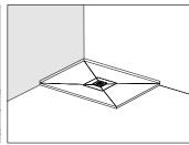
TRAY & SKIRTING INSTALLATION Tray and skirting. Remaining floor area must be built up to the same level as the base.
