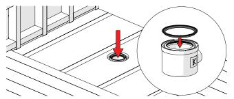
Connect waste body using 1%''/42mm UK solvent weld waste pipe (not supplied), ensuring that the waste body is positioned to centre of the cut-out.
