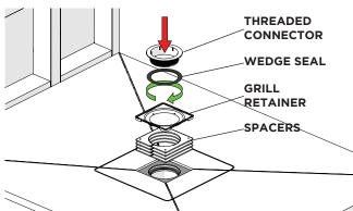
Place tray into position. Fit the Threaded Connector, Wedge Seal, Grill Retainer and Height Spacer(s). Twist the Threaded connector into the Waste using the tool provided. This will tighten and secure tray to waste.
