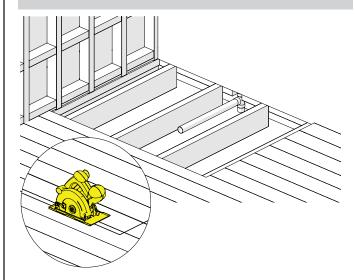
Carefully cut out the marked area on the floorboards with the Circular Saw. Be careful not to cut away at joist underneath. Ensure pipework is installed.
