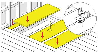
Cut 18 ply-board down to suit the spaces. Place them on top of the battens and screw into place using drywall screws.
