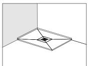
TRAY & SKIRTING INSTALLATION Tray and skirting. Remaining floor area must be built up to the same level as the base.
