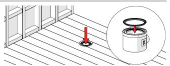
Connect waste body using 1%''/42mm UK solvent weld waste pipe (not supplied), ensuring that the waste body is positioned to centre of the cut-out.
