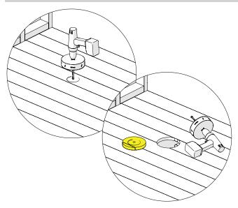
Remove the tray. In the centre of the marked position drill a hole with the Hole Saw 152mmOD, as shown. See section 2b. for solid floors.
