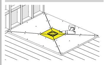
Secure the tray in place using drywall screws around outside of the square groove (indicated yellow), so that you miss the Square Steel Support Plate.
