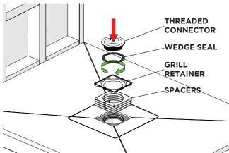
Place tray into position. Fit the Threaded Connector, Wedge Seal, Grill Retainer and Height Spacer(s). Twist the Threaded connector into the Waste using the tool provided. This will tighten and secure tray to waste.
