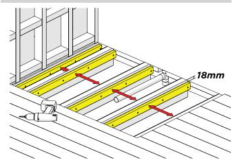
Cut down battens to suit space. Measure 18mm from the top of the joists and mark. Secure the battens in place using drywall screws, so that battens top surfaces are set 18mm below the joist top surface.
