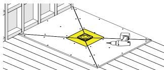
Secure the tray in place using drywall screws around outside of the square groove (indicated yellow), so that you miss the Square Steel Support Plate.
